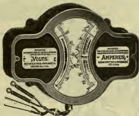
FIG. 414.—Weston Volt-ammeter of the Type used on Electric Vehicles. Other makes of these instruments have the index scales side by side, instead of end to end.
